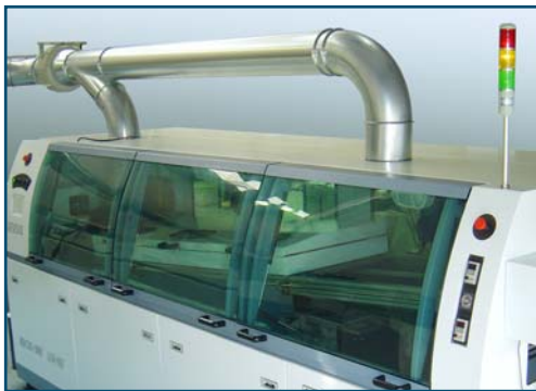
▲ Texmate's lead-free wave soldering machine
